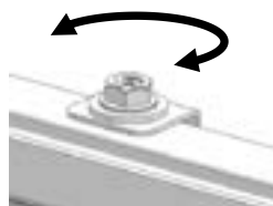
Fixing furniture door completely
